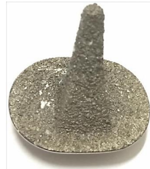
Figure 3. Wear and spalling of coating materials from surface.
