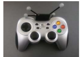
Logitech gamepad modified as input device for virtual environments with optical tracking
