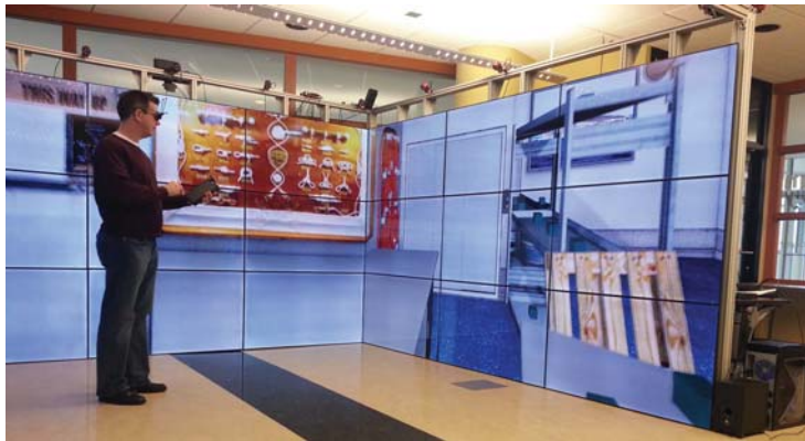
Display environment showing a virtual scenario of a room setup on an aircraft carrier getting controlled via a 7 inch tablet computer
